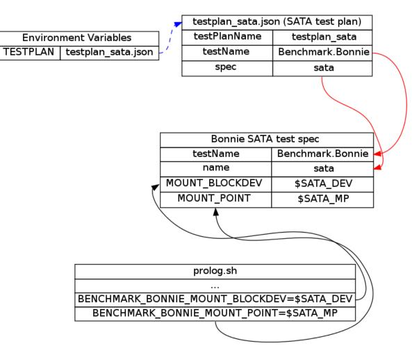
Figure 4: Simple testplan example
