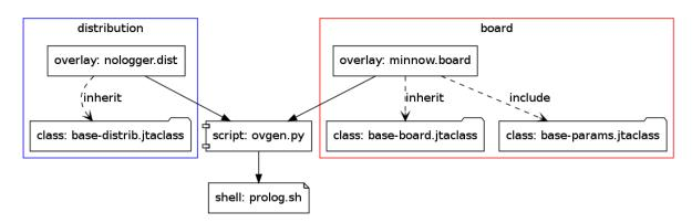
Figure 2: Fuego Base classes and overlays from toplevel perspective
